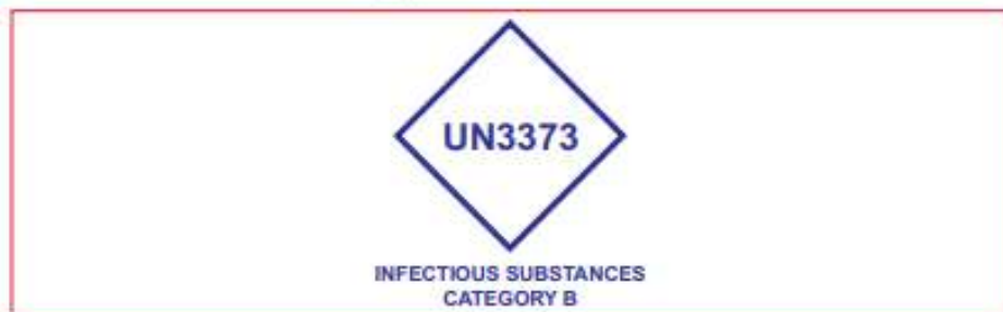
Figure 6: The marking used for the transportation of infectious substances category B
